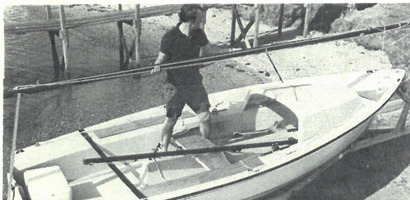
1. Mast rides securely on trailer support and boom crotch.
